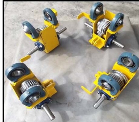
Housing Box Gear
