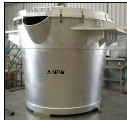
HEAT TREATMENT FURNACE
