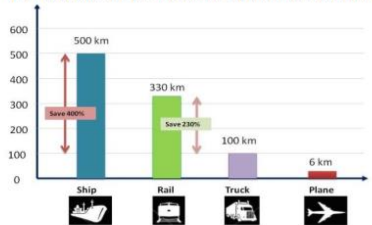
Transport distance per mode with equal fuel consumption
